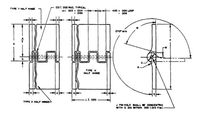
FIGURE 1. Butt hinge.
